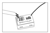
Power up the receiver by turning on the electronic speed control (electric cars) or turn on the battery switch (gas car). Note that the LED will flash continuously indicating that the receiver is ready to bind.
