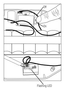
With the throttle and the steering channels set to the desired failsafe positions, (normally neutral steering and slight brakes) press and hold the bind button on the back of the module while turning on the transmitter.
