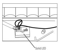
Remove the bind plug before using the system.
