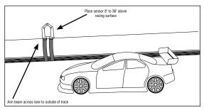
The lap trigger should be mounted 8" to 36" above the racing surface facing outward from the track. Facing the trigger outward keeps the IR beam from crossing the track in more than one lane preventing unwanted false triggering. Hook and loop strips make mounting easy. Only one lap trigger is necessary at each track, as a single infrared beam will trigger the lap timer in all cars.
