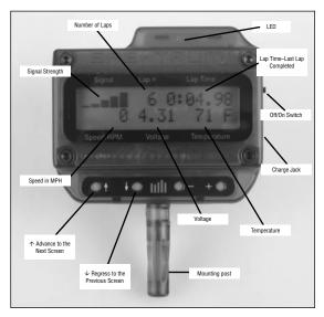
Note: Two sizes of mounting posts are provided. This allows the handheld unit to be mounted in different antenna holes.
