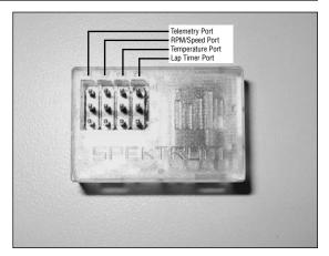
The telemetry module is used to interface the sensors to the receiver (transceiver). The module is attached to the receiver via the included male-to-male telemetry lead provided. The telemetry lead must be plugged into the BAT/TEL port in the receiver and into the T battery port in the module. See photo of receiver and telemetry hooked up with cord.
