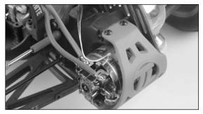
Plug the temperature sensor into the port marked E in the telemetry module. The handheld unit should now display room temperature.
