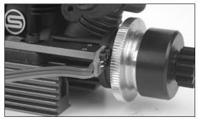
If the flywheel is reflective (bare metal), place a flat black decal on the flywheel so it passes between the sensor and the flywheel when rotated.
