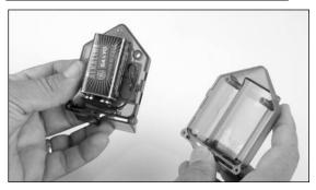
Use 3/32" and 5/64" hex wrenches to unscrew the case and install the 9-volt battery as shown. Reinstall the case, being careful not to over-tighten the screws.
