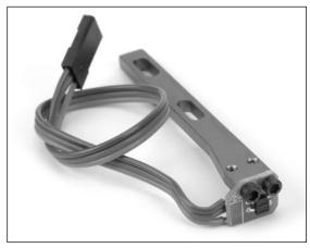
Install the mount under the engine screw and adjust the sensor so it is 1/8" from the flywheel.
