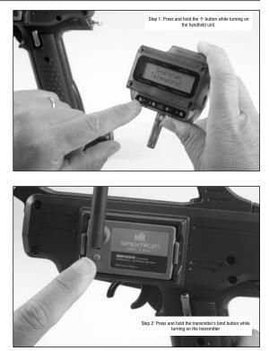
It is necessary to bind the handheld unit to the transmitter. Binding teaches the handheld unit the specific code of the transmitter and when bound, the handheld unit will only listen to information coming from the receiver(s) that are bound to that transmitter. To bind the handheld unit:
