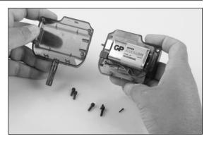
Using a 3/32" and .050" hex wrench, unscrew the case and install a 9-volt battery as shown.
