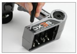
4. Separate case halves, being careful with antenna and wiring. Set back half of case aside.
