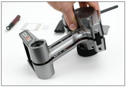
5. Carefully pull out rolling selector circuit board.
