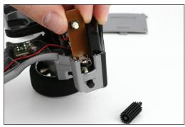
6. Remove broken rolling selector and pin inside the wheel encoder.
