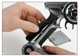
2. Carefully remove the top label and LCD cover being careful not to scratch the LCD.
