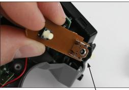
Be sure the broken pin is removed.
