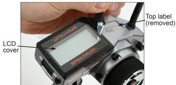
3. Remove 9 case screws. **Note:** One screw is behind the bottom label.
