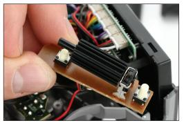
8. Replace rolling selector circuit board. Be sure the board aligns with the tracks in the case. Also, be sure the small black button is still in place.
