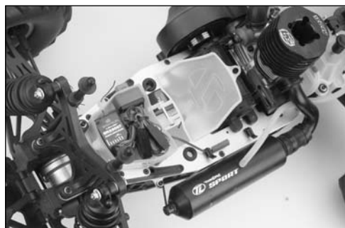
Typical Gas Installation
