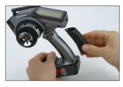
14. Fit the grip in place and reinstall the batteries.
