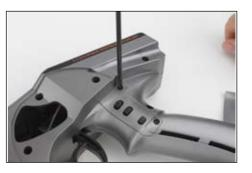
9. Place both grip plates in place and fasten them using four Phillips screws (two per side).
