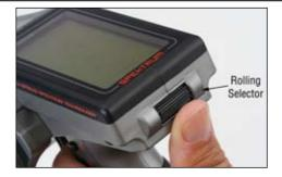
The Rolling Selector is pressed to access functions and rolled to select specific features or to change settings or values. Pressing and holding the rolling selector for more than three seconds returns the display to the main screen.
