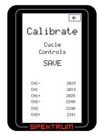
Rotate the steering wheel full right then full left; then move the throttle trigger to full throttle and full brake.
