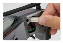
10. Push the steering wheel connector through the transmitter case to the opposite side.
