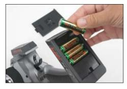
1. Remove the batteries from the transmitter. This prevents the possibility of accidentally causing a short during the conversion.
