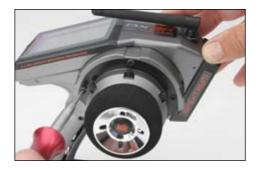
3. Using a 3/32-inch hex wrench, remove the three screws on the front of the steering housing as shown.
