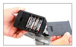
Remove the battery door and install 4 AA batteries, noting that the polarity of each corresponds with the diagram in the battery holder. Replace the battery door.
