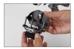
11. Select the opposite "handed" steering shell and pass the steering wheel mechanism connector through the hole in the shell.
