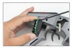
6. Carefully pull out the grip plate that contains buttons D, E and F. Using a Phillips screwdriver remove the PC board and backplate from the grip plate. Note the positions of the three buttons.
