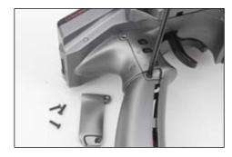
5. Using a small Phillips screwdriver, remove the four Phillips screws (two per side) that fasten the grip plates in place and remove the grip plate that doesn't have the buttons attached.
