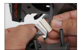
12. Connect the steering wheel mechanism connector to the connector from the transmitter being sure the connection is tight. Note correct polarity.
