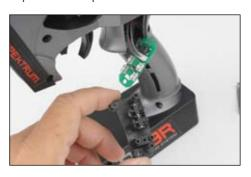
7. Transfer the three buttons (D,E and F) to the other "handed" grip plate noting that the buttons fit in a specific direction so that they fit the external contour of the grip plate.
