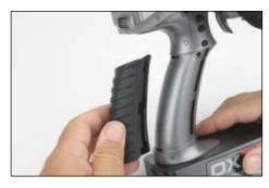
2. Carefully remove the grip cover by prying with your fingers at the forward edge of the rubber grip.
