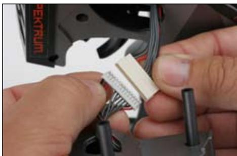
12. Connect the steering wheel mechanism connector to the connector from the transmitter being sure the connection is tight. Note correct polarity.
