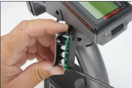
8. Carefully screw the PC board and backplate in place and test that all buttons are depressing properly.
