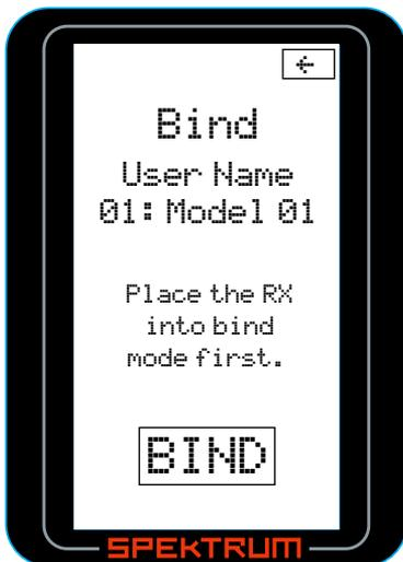
6. Rotate the roller to highlight BIND.
