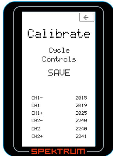
Rotate the steering wheel full right then full left; then move the throttle trigger to full throttle and full brake. Note: The values will change to correlate with the actual potentiometers.
