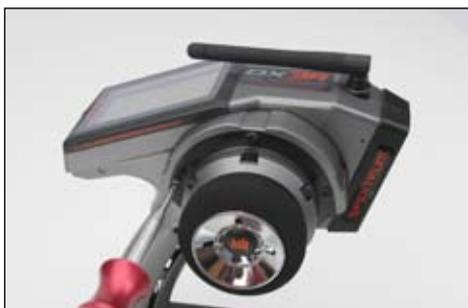
13. Fit the other handed backplate in place and secure the steering wheel assembly in place using the three long cap head screws.
