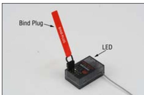
**Note:** The SR3100 features DSM2 second-generation technology and is only compatible with transmitters that utilize DSM2 protocol (like the DX3R). DSM1 transmitters will not use the SR3100 receiver.
