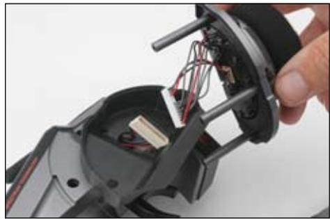
4. Carefully remove the steering mechanism and unplug the steering connector. Also remove the backplate.
