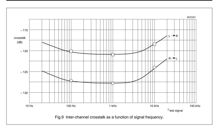
**Note:** Graph constructed from average measurements values of a small amount of engineering samples. No guarantee for typical values is implied.
