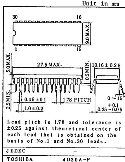
Lead pitch is 1.78 and tolerance is ±0.025 against theoretical center of each lead that is obtained on the basis of No.1 and No.30 leads.
