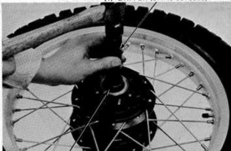
(2) ATTACHMENT, 37 x 40 mm (07746-0010200) AND PILOT, 17 mm (07746-0040400)
